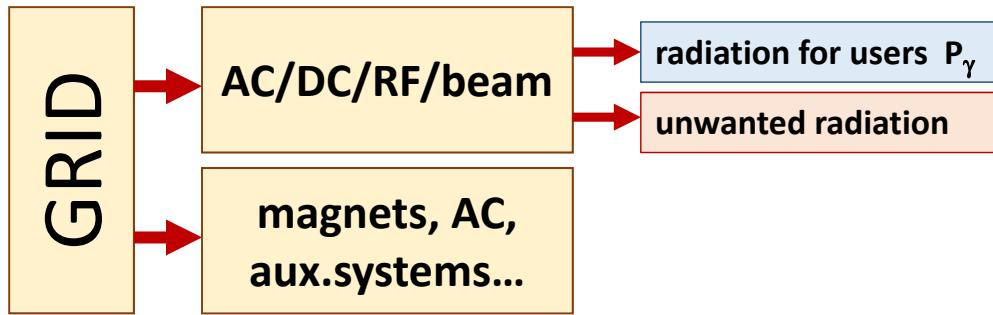
efficiency figure:  $\eta_{\text{total}} = \frac{P_{\gamma, \text{users}}}{P_{\text{grid}}}$
