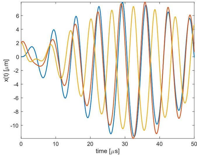
**Simple numerical example:** nonlinear simple harmonic oscillator with time-varying initial conditions, inputs, and parameters.
