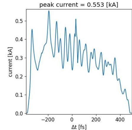
Bunch compression amplifies small time-varying perturbations in initial beam distributions.
