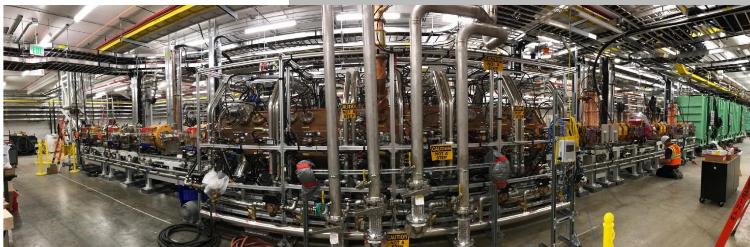
FRIB Lower LEBT, RFQ, MEBT, and the three  $\beta=0.041$  cryomodules
