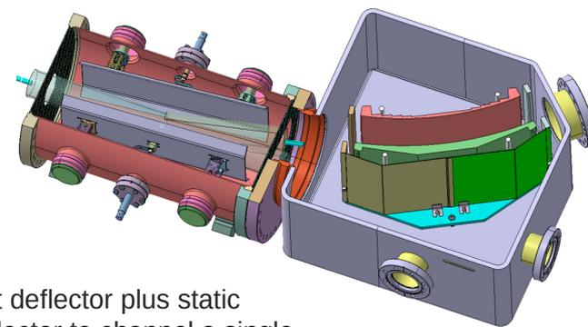
fast deflector plus static deflector to channel a single bunch towards a different line
