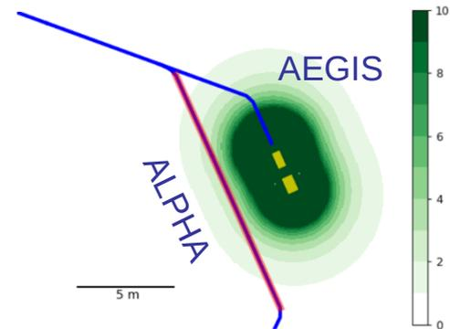
1 G.m of transverse integrated magnetic field induces a deviation of around 2 mrad
