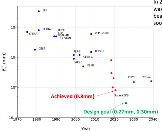
In 2022b run, we tried  $\beta y^*=0.8$ mm. The specific luminosity was higher than  $\beta y^*=1$ mm case. We could not store higher beam currents due to poor injection efficiency. We will re-try
