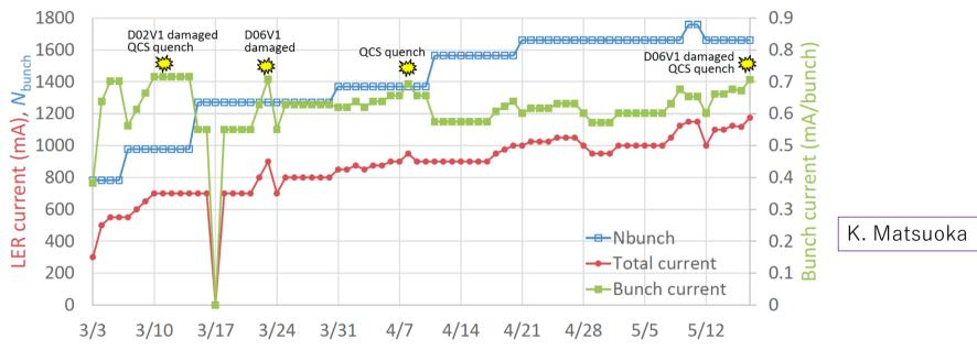
The three big accidents of LER beam loss in 2022 happed at  $I_b > \sim 0.7 \text{mA/bunch}$  within a day after increasing the beam current at the three different  $N_{bunch}$  -> Empirical rule: we must not exceed 0.7 mA/bunch.
