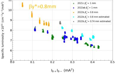
In the data in cyan and blue, estimated values of  $\beta y^*$  in HER were less than 1mm(setting value) due to horizontal orbit change in SLY depending on total beam current.
