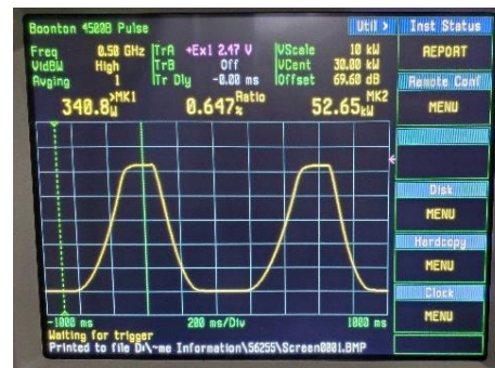
Figure 5: Booster ramping. Yellow: RF envelope.
