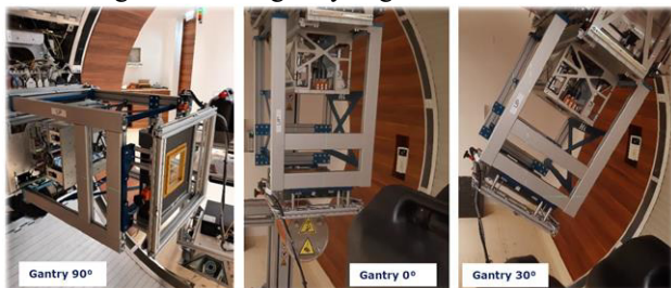
Figure 6: Beam commissioning: beam monitor mounted on holder frame in the gantry room at different gantry angles.
