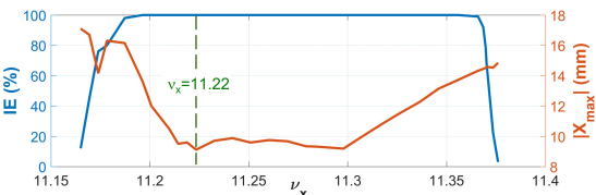
Figure 6: Horizontal tune and its effect on residual oscillations and injection efficiency.
